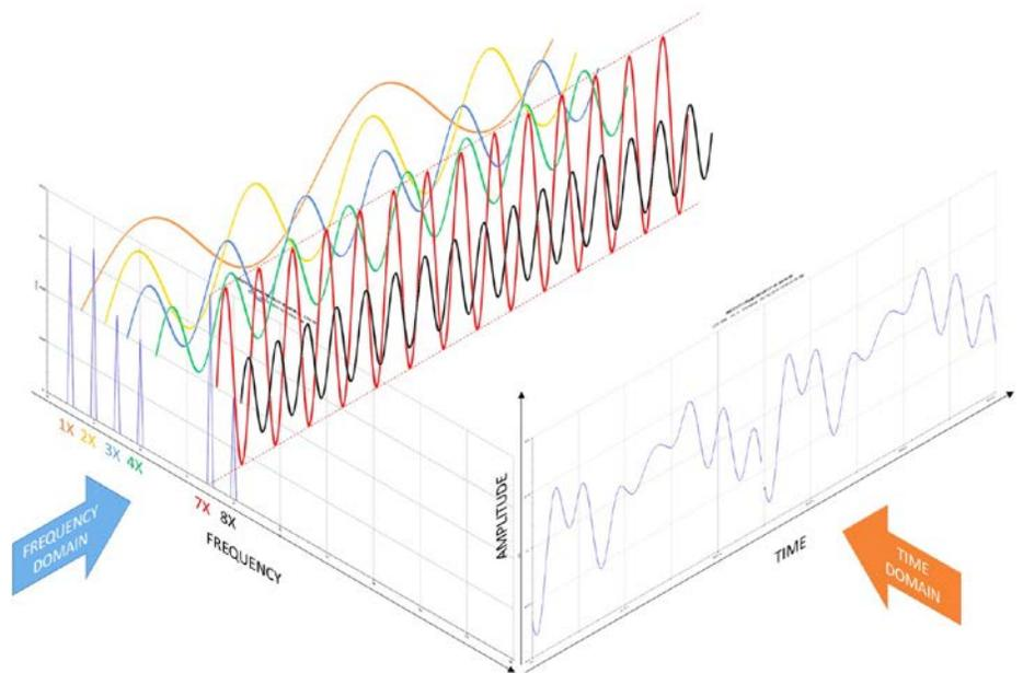
**Figure 1:** Vibration waveform showing relationship between time and frequency domains.
