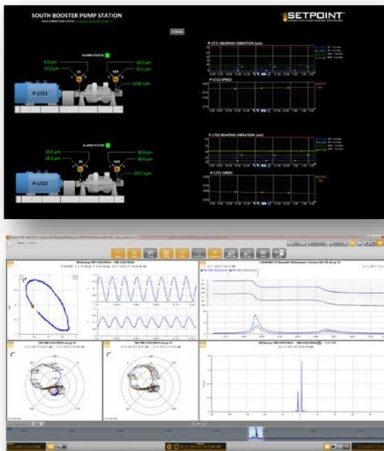
*The PI System can be used to deliver not just the things you're used to seeing like trends and current values (top), but also vibration waveforms in all of the specialized plot formats (bottom) used by rotating machinery engineers.*
