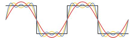
**Figure 2:** Fourier series approximation of a square wave when one (red), two (yellow), and three (blue) harmonics are included. Notice that the 1X component (red) has an amplitude that is larger than the direct (black) value.
